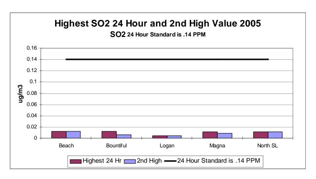
The following graph shows the history of SO<sub>2</sub> concentrations measured in Utah. The graph shows the last time the standard was exceeded was 1981. Since that time SIP requirements and control measures implemented by industrial operations have resulted in low SO<sub>2</sub> levels.
